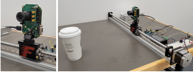
Fig. 2. Experimental setup with Prophesee Mk3 event camera on a motorized linear rail. The rail is programmed to translate the camera a short distance to capture different viewpoints along a plane to form the EPIs.
