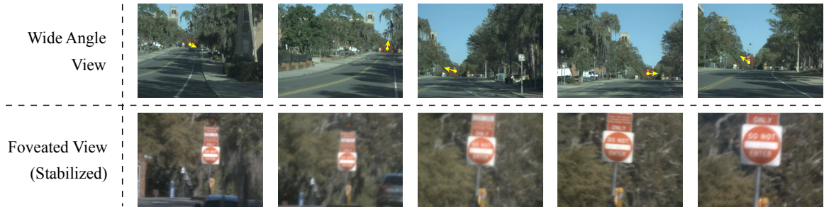
(c) Stabilization on a traffic sign with the camera mounted on a vehicle driving towards it. The sign stays in the center of fovea FOV even when driving over speed bumps.
