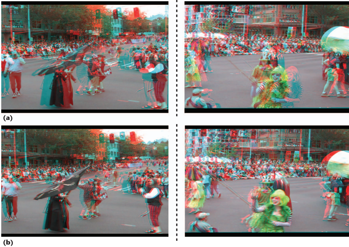
Figure 12. Easing the transition between two clips by crossfading the horizontal image translation to zero at the cut. (a) A direct transition. (b) Cross-fading the horizontal image shift.
