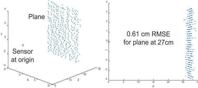
(III) Validation by reconstructing a plane at 27cm
