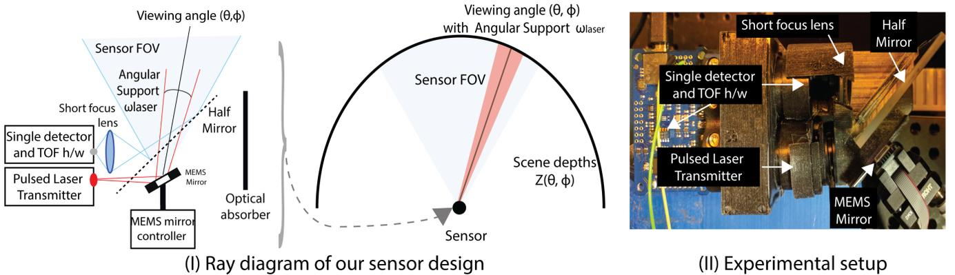
Fig. 1. Ray diagram: In (I) we show the co-located ray-diagram of the pulsed LIDAR that is modulated by a MEMS device. In (II) we show our actual setup, with a Lightware LIDAR and a Mirrorcle MEMS mirror.
