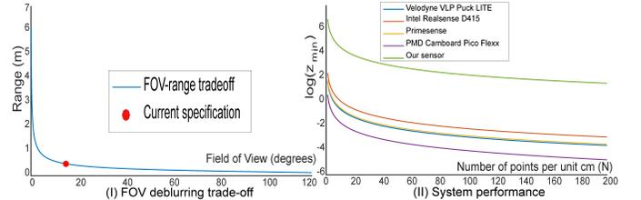
Fig. 8. In (I) we depict the deblurring trade-off in our setup, where increasing FOV results in reduced SNR and range. In (II) we compare our LIDAR zoom to other available depth sensors which have fixed acuity.
