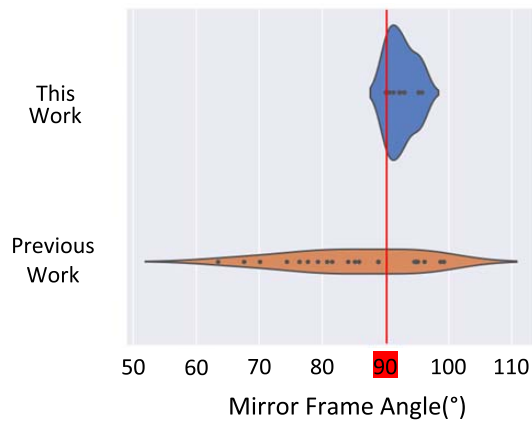
Fig. 8. A comparison between the sample distribution of the measured mirror frame angles from this work and the previous works.
