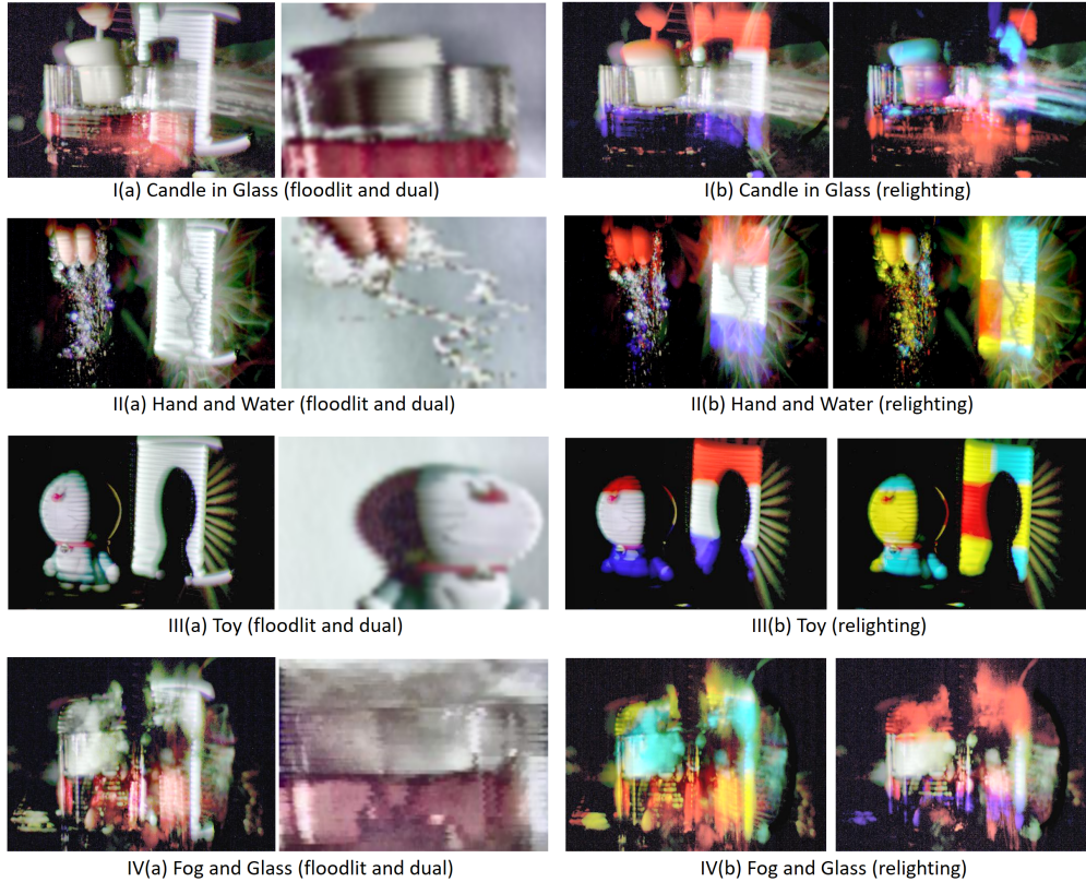
Fig. 2. Real Line-of-sight results. Here we show floodlit, dual and relighting results for four dynamic scenes. Please see the supplementary video. In (I) we show a wax candle placed in a liquid-filled cup. In (II) we show water droplets falling off fingers. In (III) we show a toy being rotated, and in (IV) we show fog-like vapors from dry-ice placed in a cup containing colored water. Note the caustics in the relighting, and the shadows/specularities maintained in the dual views.
