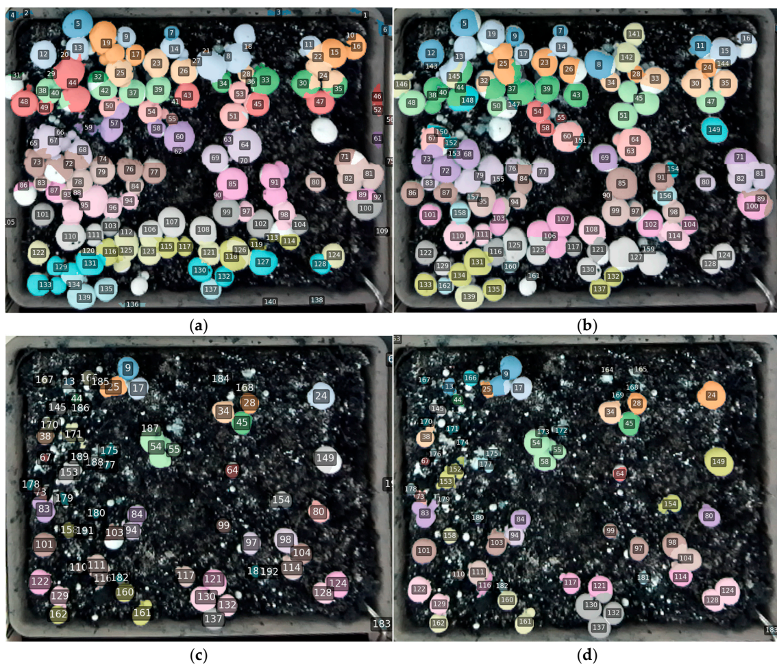
Figure 15. Example of RD-GuideNet-based multi-frame tracking of white-button mushrooms across sequential frames within the same bed. (a) Initial frame showing assigned track IDs; (b) frame captured 10 min later, where most mushrooms retain identical IDs despite minor changes in cap size, pose, and local crowding, demonstrating robust temporal association; (c,d) frames acquired post-harvest, where IDs corresponding to removed mushrooms are absent, while remaining mushrooms preserve their prior identities. The consistent color-coded IDs and well-preserved boundaries confirm RD-GuideNet’s ability to maintain long-term identity continuity, even under occlusion and partial harvesting.
