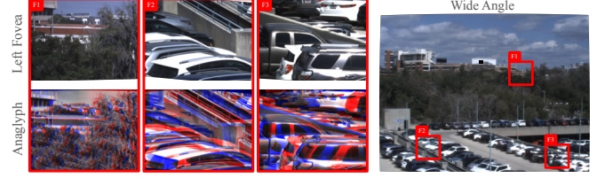
Fig. 11: Visualization of one collected scene of the rasterized dataset. For each scene, a wide-angle shot is captured alongside 81 pairs of foveated images. Here we show the left fovea image capture, the anaglyph between the left and right fovea image, and the wide-angle capture.
